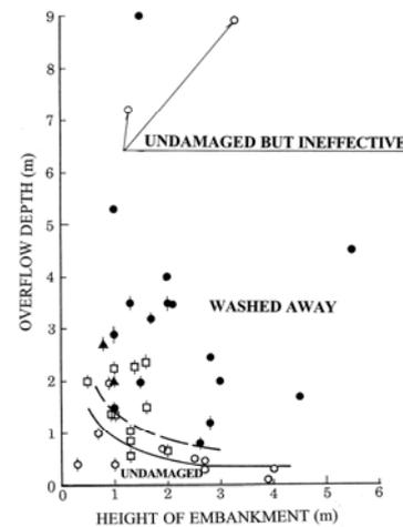
Fig.5 Damage to embankment
