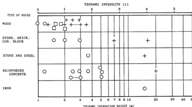
Fig.3 Damage to houses. Circles; withstand. Squares; partially damaged. Crosses; Washed away.
